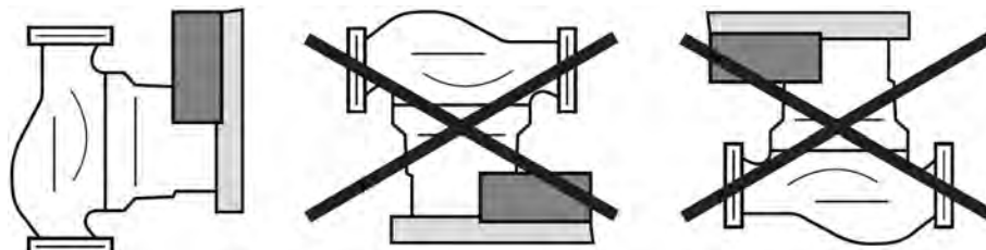
Wet-motor pump installation ver. 1
